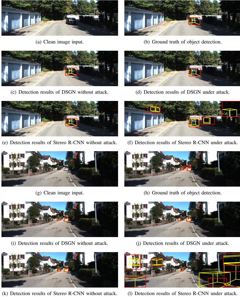
Fig. 2. When there is no attack, both Stereo R-CNN and DSGN can detect objects accurately as shown in (c), (e), (i), and (k). When the perturbation attack is launched, the two models produce erroneous object detection results including inaccurate detection of real objects in (d), (j), and false detection of ghost objects in (f), (l).
