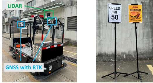
(a) Testbed car equipped with LiDAR and GNSS. (b) Cardboards affixed to tripods.
